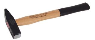
Features & Benefits  $\sim$  According to DIN 1041  $\sim$  Traditional ash shaft, lacquered  $\sim$  Grip section with textured non-slip laquer  $\sim$  Head secured by ring wedge and epoxy resin  $\sim$  Head length: 80 mm  $\sim$  Overall length: 260 mm  $\sim$  Weight: 100 g
